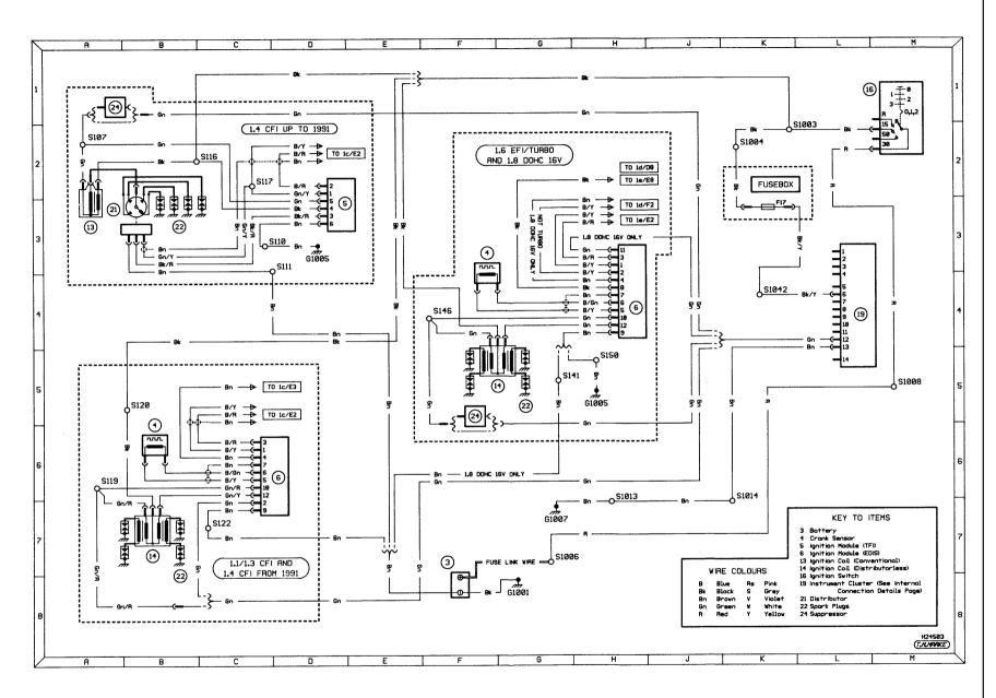
Diagram 1b: Ignition system - fuel-injected models
